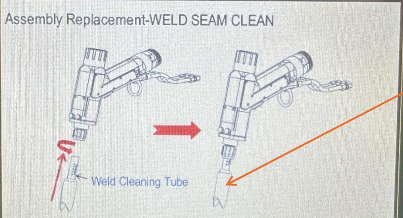
Remove the wire feed assembly, remove the extension tube, and replace the cleaning tube in the direction shown in the illustration. Then tightly lock the cleaning tube in the direction of rotation.
