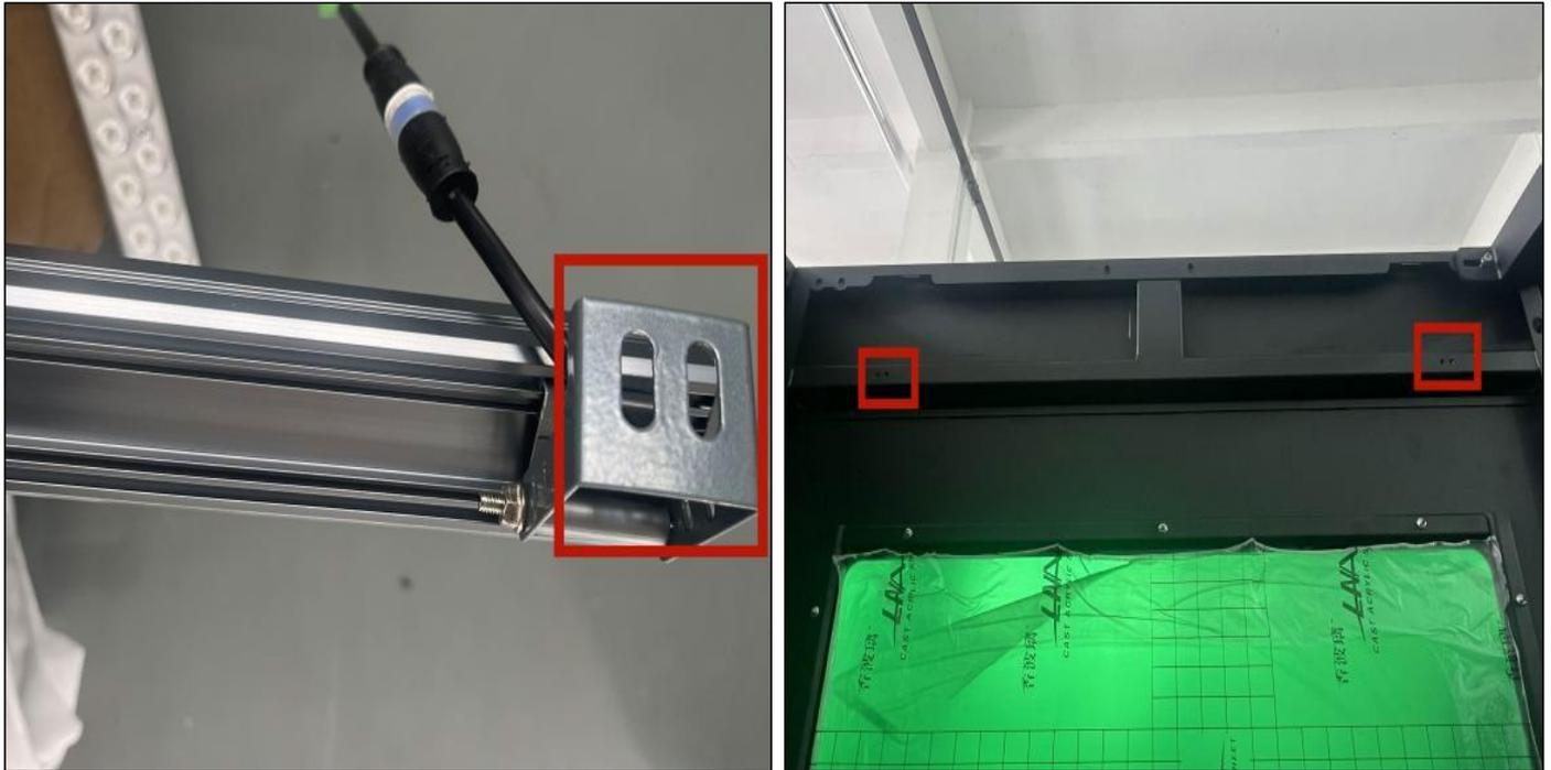
The diagram below shows, where the lamp post connection begin, The front and back sides are fitted with lamp posts, four in total, connected to each other as in the picture below.
