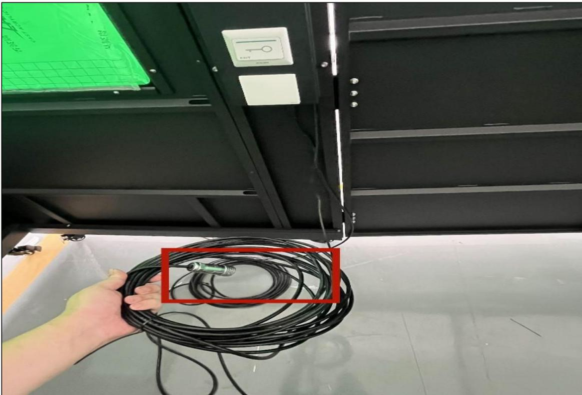
The following diagram shows the 220-volt power connection cables that are supplied to the lampposts,access control unit.
